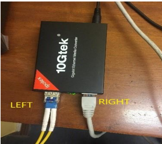
Fig. 2: Electrical-to-Fiber or Fiber-to-Electrical Converter
