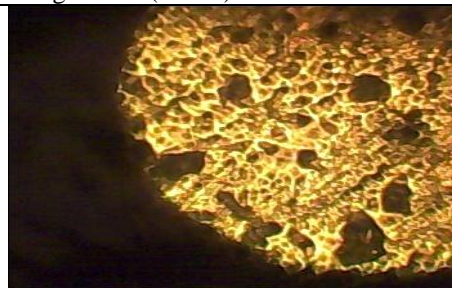
Plate 7. Micrograph of specimen subjected to heat input of 2.12kJ/mm using E7018 (X 400)
