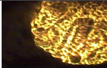
Plate 2. Micrograph of specimen subjected to heat input of 1.53kJ/mm using E6013 (X 400)
