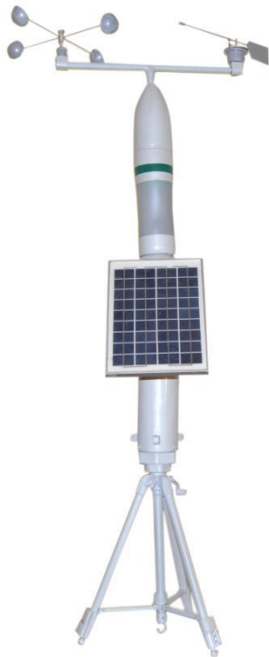
Figure 4: Constructed weather station
