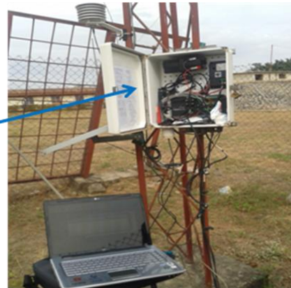
(b) Downloading of Atmospheric Data to a Laptop
