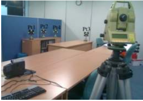
Fig. 1: Deformation monitoring experiment
