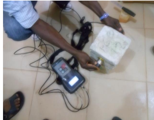
Figure 2 Testing using UPV machine
