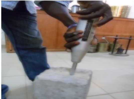
Figure 2 Testing using schmidt rebound hammer
