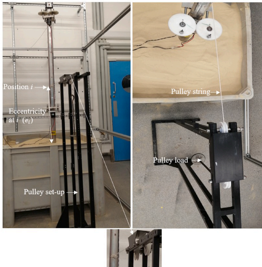
Fig. 8. Ultimate (pure) moment capacity test set up of the LOWT model.
