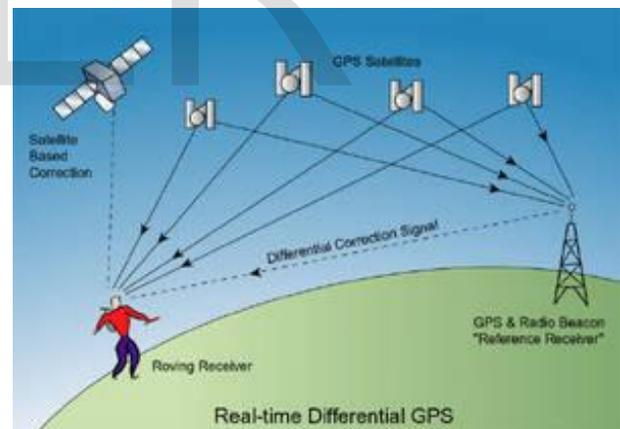
Fig. 1: GPS Signal Propagation between Satellite and User Segments [3]
