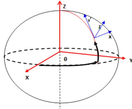
Fig. 2: The WGS-84 Geocentric Cartesian Coordinate Reference Frame ( $X, Y, Z$ ) used by GPS and Local Level Coordinate Reference Frame ( $x', y', z'$ ).
