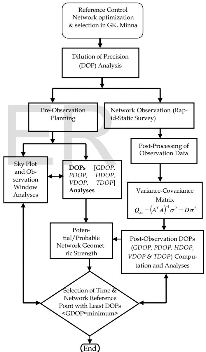
Fig. 5: GPS Ground Control Reference Network Optimization and Selection Algorithm for Gidan Kwano Area of Minna, Nigeria
