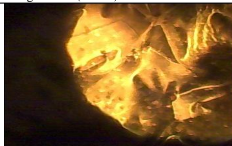
Plate 9. Micrograph of specimen subjected to heat input of 1.22kJ/mm
