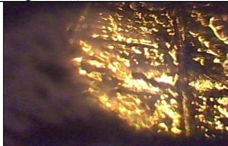
Plate 4. Micrograph of specimen subjected to heat input of 0.88kJ/mm using E6013 (X 400)
