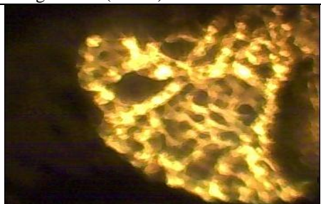
Plate 8. Micrograph of specimen subjected to heat input of 1.22kJ/mm
