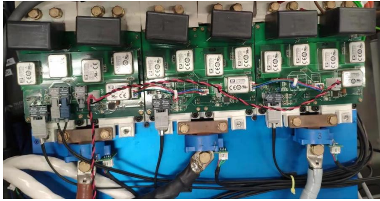
Figure 8. A three-level converter developed in the University of Nottingham within Clean Sky AEGART project
