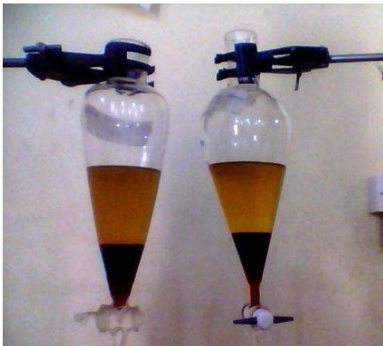
Plate 2: Biodiesel settling stage before glycerol removal
