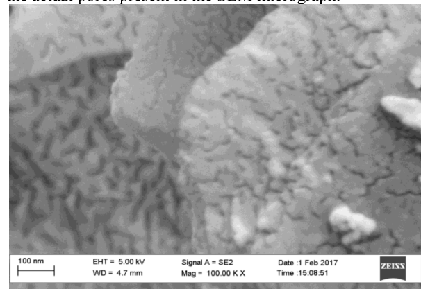
Figure 6(a): SEM of KCl Activated Carbon at 100,000X (in nm)
