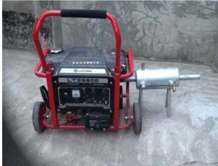
Fig. 2. The gasoline generator coupled with heat exchanger
