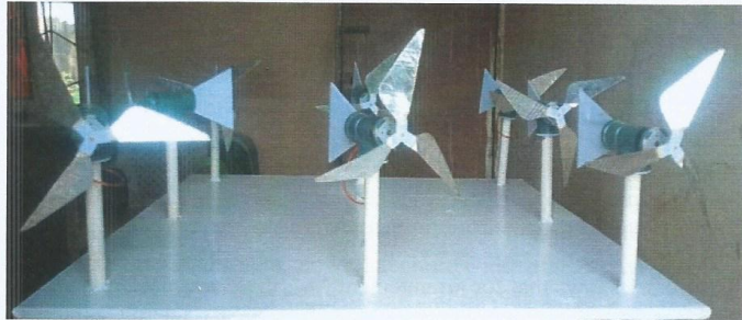
Figure 2.17: Assembled micro-wind turbine charger
