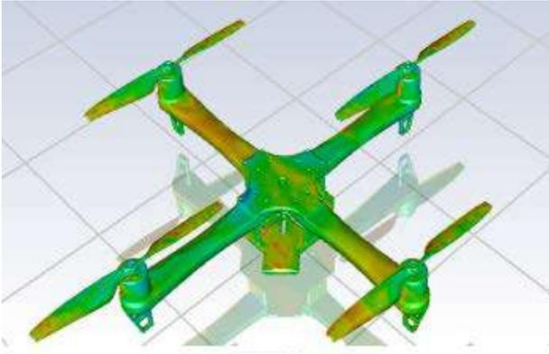
**Fig. 8:** Total surface pressure flow simulation result
