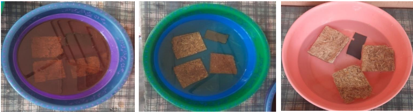
Figure 4: Samples being wholly immersed in engine oil, petrol and water respectively
