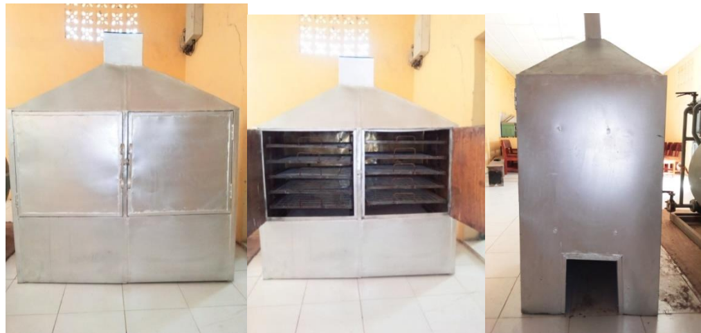
Plate 3: Fabricated NIFFR Improved Smoking Kiln
