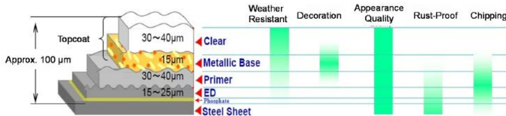
Figure 1: Automotive Coating Layers, thicknesses and purposes for An exterior Surface (Nelson et al, 2016).
