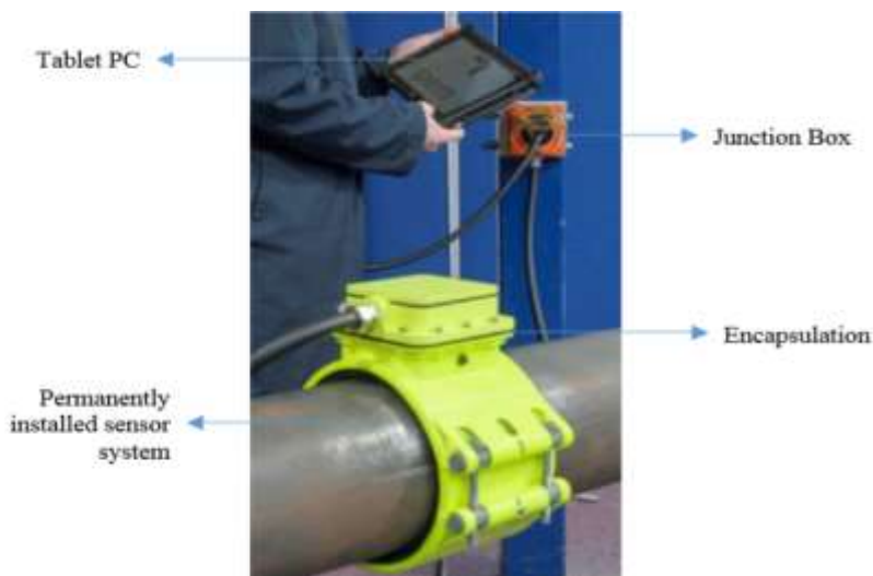
Figure 9: iPerm System Hardware Components [17]
