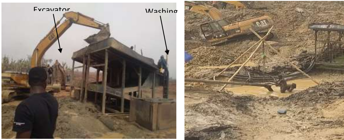
Figure 2: Excavator loading the washing pan
