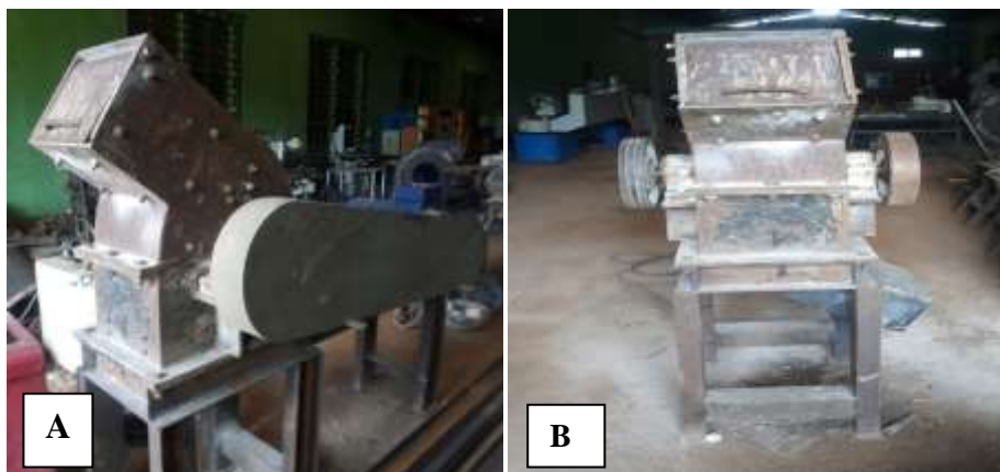
Fig. 8: The complete hammer Crusher assembly (A-side view; B-front view)
