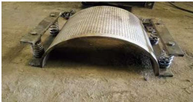
Fig.4: The screen incorporated with helical springs
