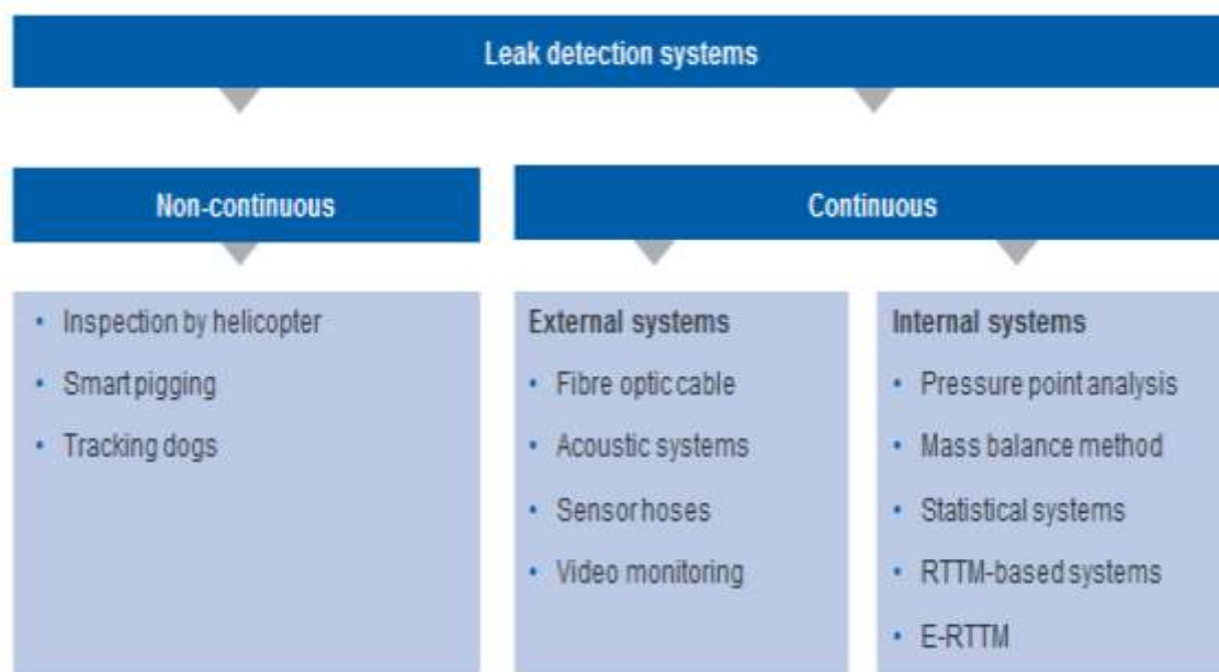
Figure 1: Summary of Leak Detection Systems [4]
