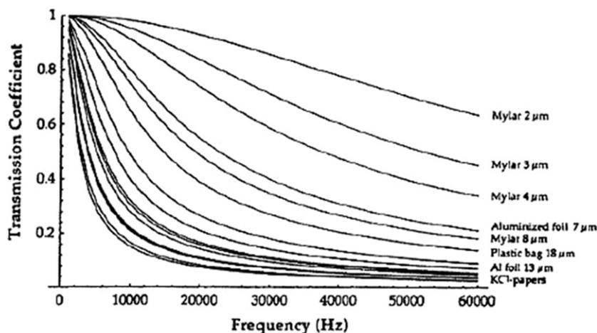
**Figure 1** The acoustic transmission vs. foil thickness according to Vuohelainen (1998). Note the excellent resolution at 2–4  $\mu\text{m}$ .
