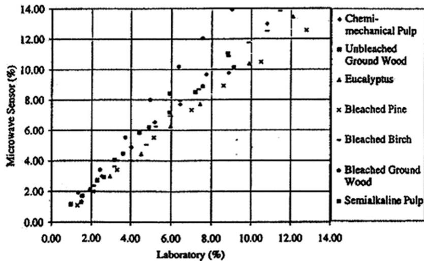
Figure 2 Consistency vs. microwave transmission.
