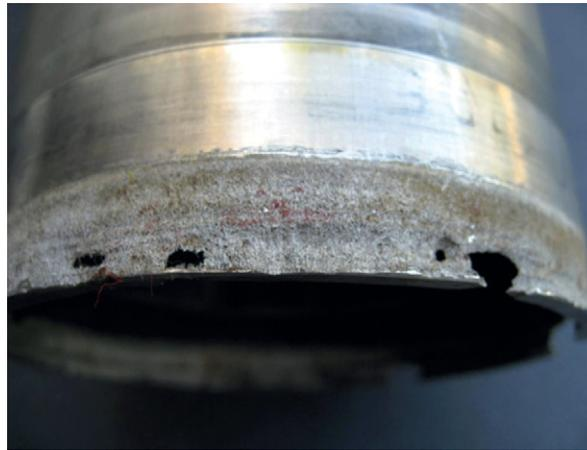
**Figure 19** Crevice corrosion of Type 316L stainless steel pump shaft sleeve in natural seawater.
