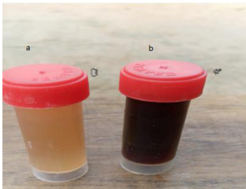
Plate 2. (a) Aqueous extract of pawpaw leaves (b) AgNPs from pawpaw leaf extract.
