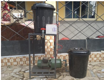
Figure 2: Prototype of smart water pump control system with remote access
