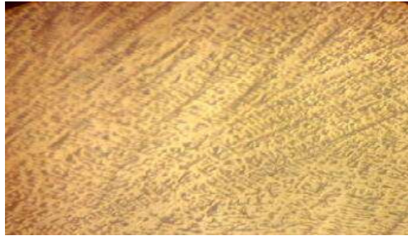
Figure 6(g): Microstructure of weld metal of TIG joint (200X)
