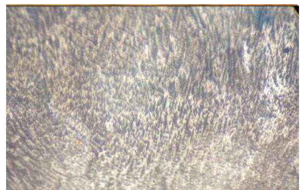
Figure 6(d): Microstructure of heat affected Zone of MMA joint (200X)
