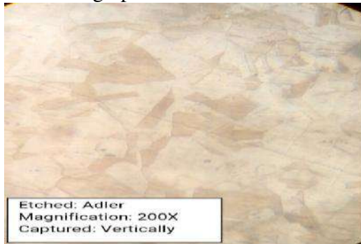
Figure 6(a): Microstructure of parent AISI304L stainless steel (200X)
