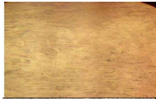
Figure 6(d): Microstructure of heat affected Zone of MMA joint (200X)
