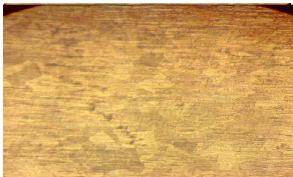
Figure 6(e): Microstructure of heat affected zone of TIG joint (200X)
