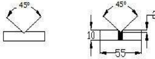
Figure 6: design of the impact test specimen
