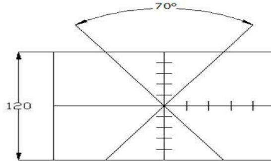
Figure 7: Design of the hardness test specimen
