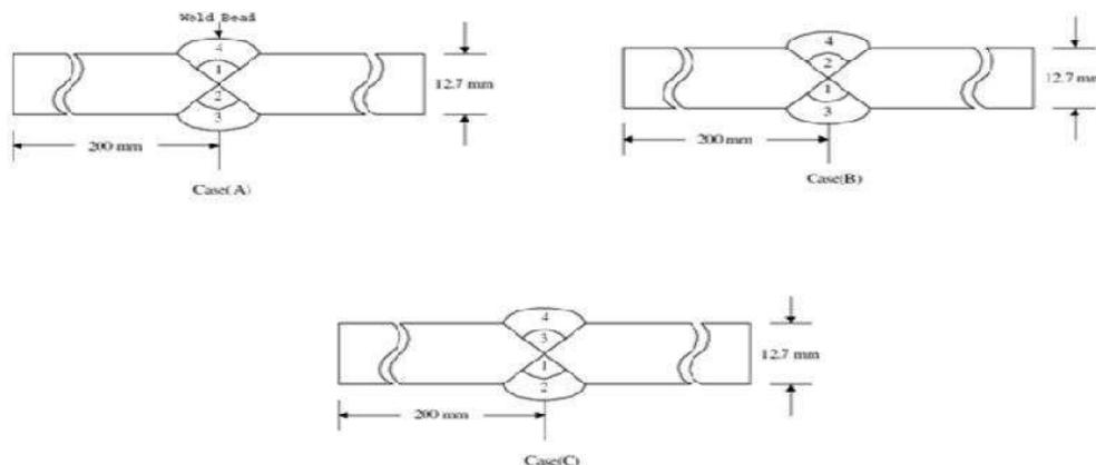
Figure 2: Different welding sequence for butt weld
