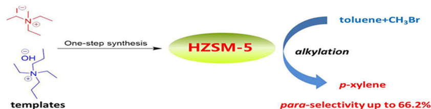
Figure 4. Dual template mechanism shape selective zeolites synthesis [137].
