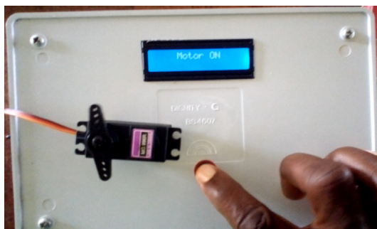
Figure d: Activation of Button, Display with Motor on and Motor Begins to Move
