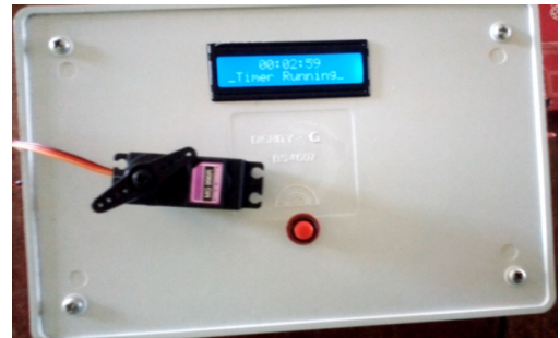
Figure e: Drive Position of Submerge Atalla Lift Net Manipulator Arms for a Catch and Count Down Display
