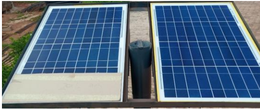
Figure 8: Normal image of 40W Polycrystalline module subjected to 20% horizontal shading.
