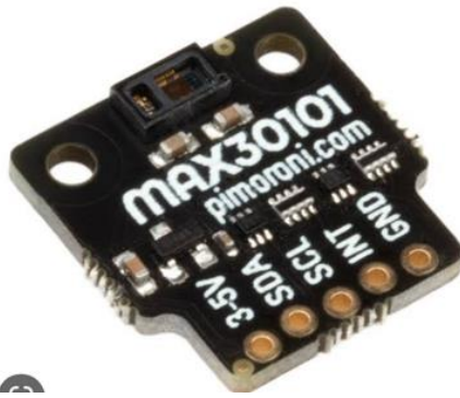
Figure 5: MAX30101 HR and BP sensor
