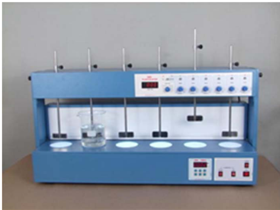
Plate 3: Jar Test Equipment (Flocculator)
