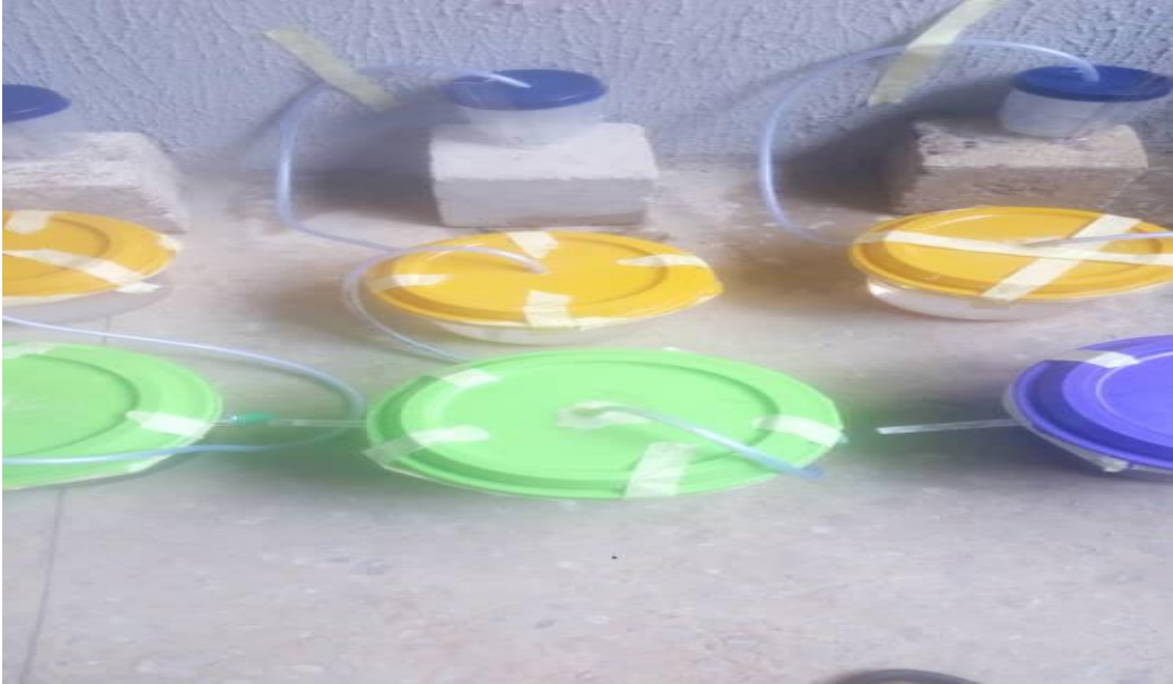
Figure 1: The Digester and the Gas Holder
