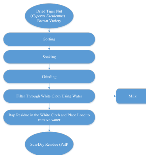
Figure 2.0: Flow Diagram for Preparation of Cyperus Esculentus Bio-Coagulant
