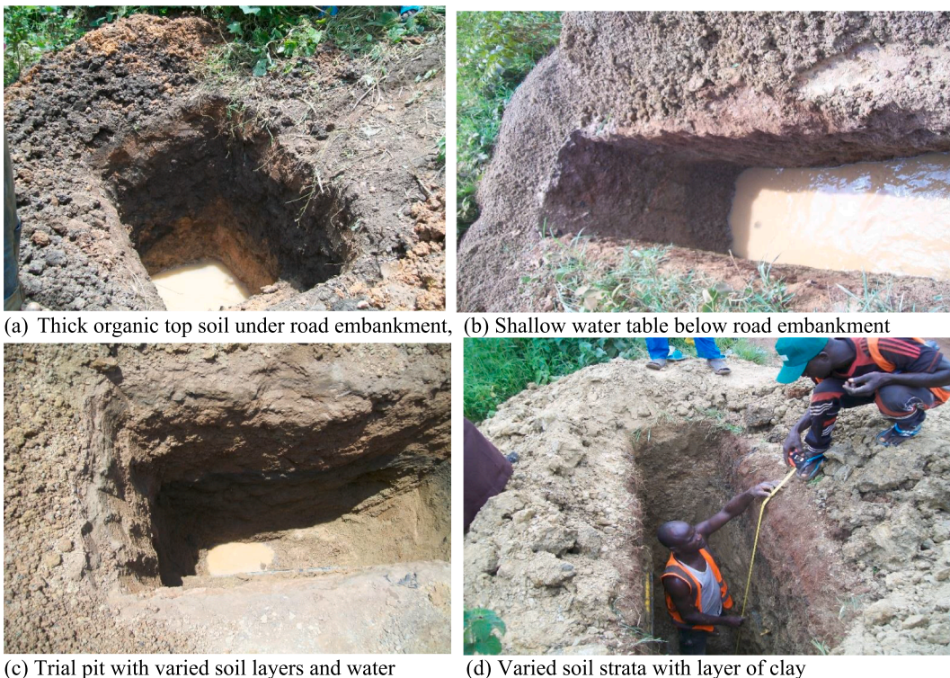
Fig. 3. Trial pit with (a) thick organic top soil (b), shallow water table, (c) varied soil layer (d) Bida basin.
