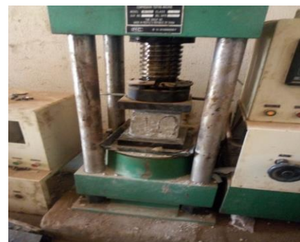
Figure 1: Specimen undergoing compressive strength test
