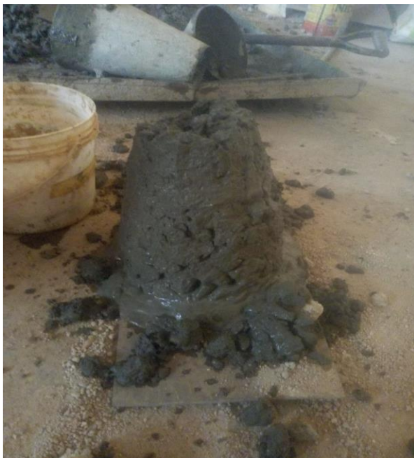
Figure 3: Sample undergoing slump test
