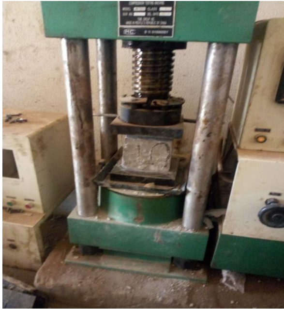
Figure 2: Sample undergoing compressive strength test
