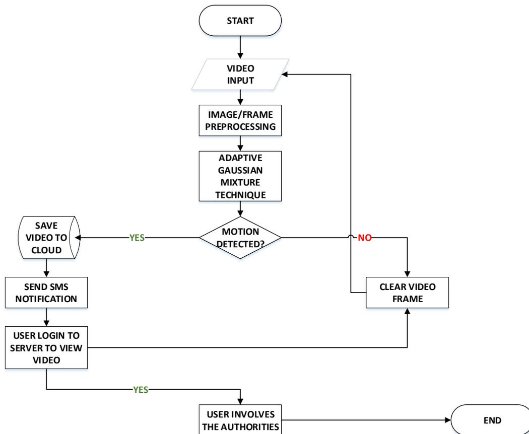
Figure 5: Flow Chart Diagram of the Developed System
