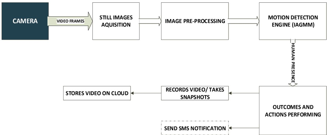
Figure 4: Data Flow Diagram of the Developed System
