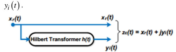
Figure 3. Conceptual Hilbert Transformer
