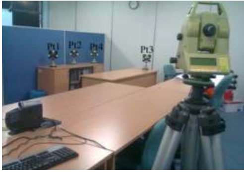
Fig. 1: Deformation monitoring experiment
