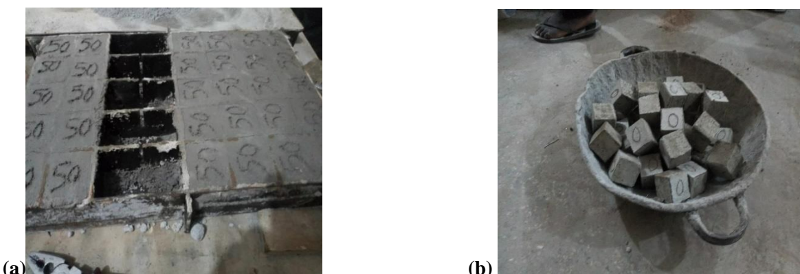
Figure 10: FHA/CCW Mortar cubes: (a) cast cubes (b) De-moulded mortar cubes
