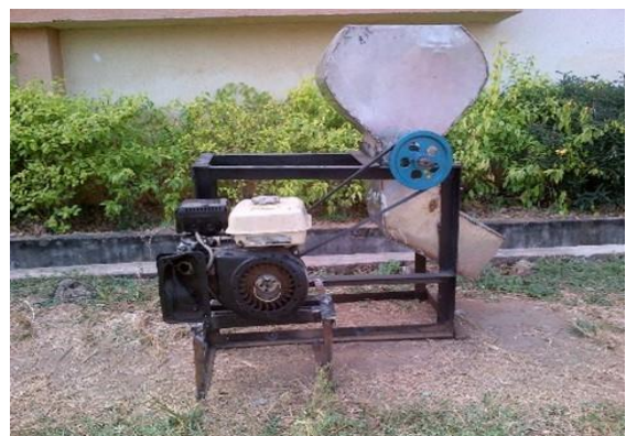
Fig. 8: Assembled cassava grater
