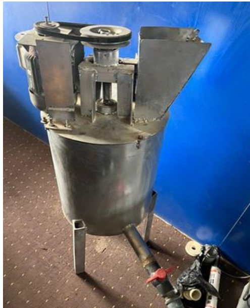
Fig. 13. Developed 50-litre batch capacity industrial mixer
