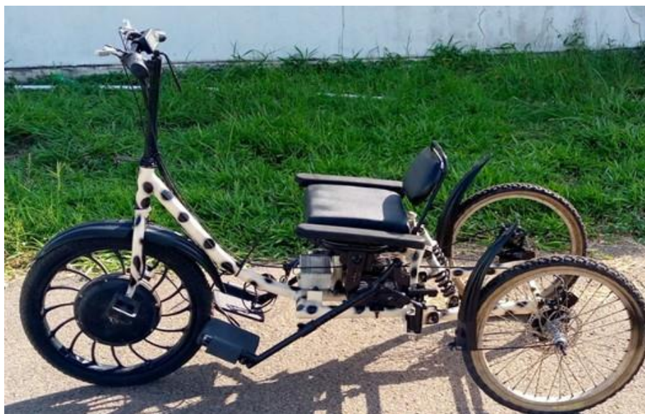
Fig. 5. Developed tricycle with adjustable wheel camber
