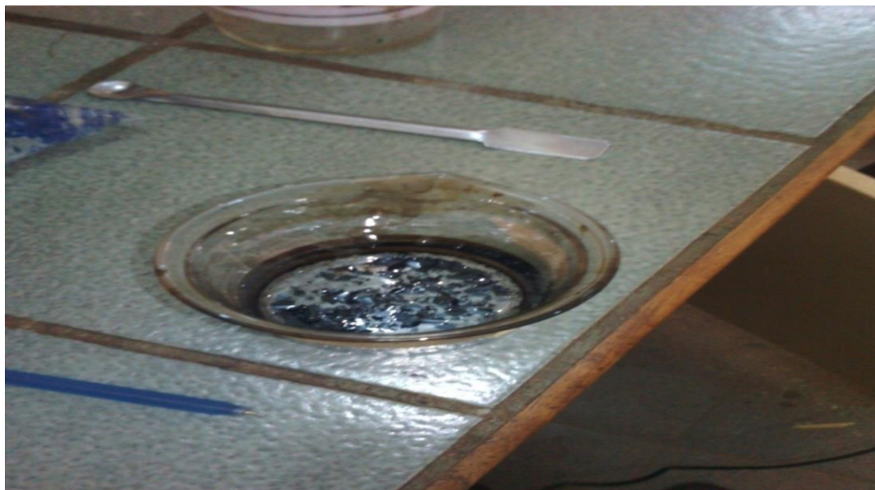
Figure 2: Showing flakes of n\text{-C}_6 asphaltenes obtained from the bitumen
