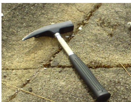
Figure 3: Jointed granite in Maikunkele area
