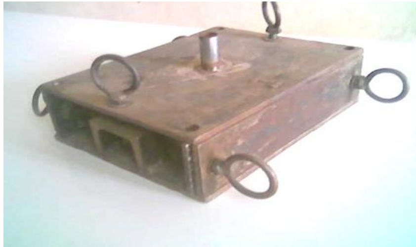
Fig. 3. A-two part mould (assembled) fabricated at danata and sawoe workshop, Abuja.
