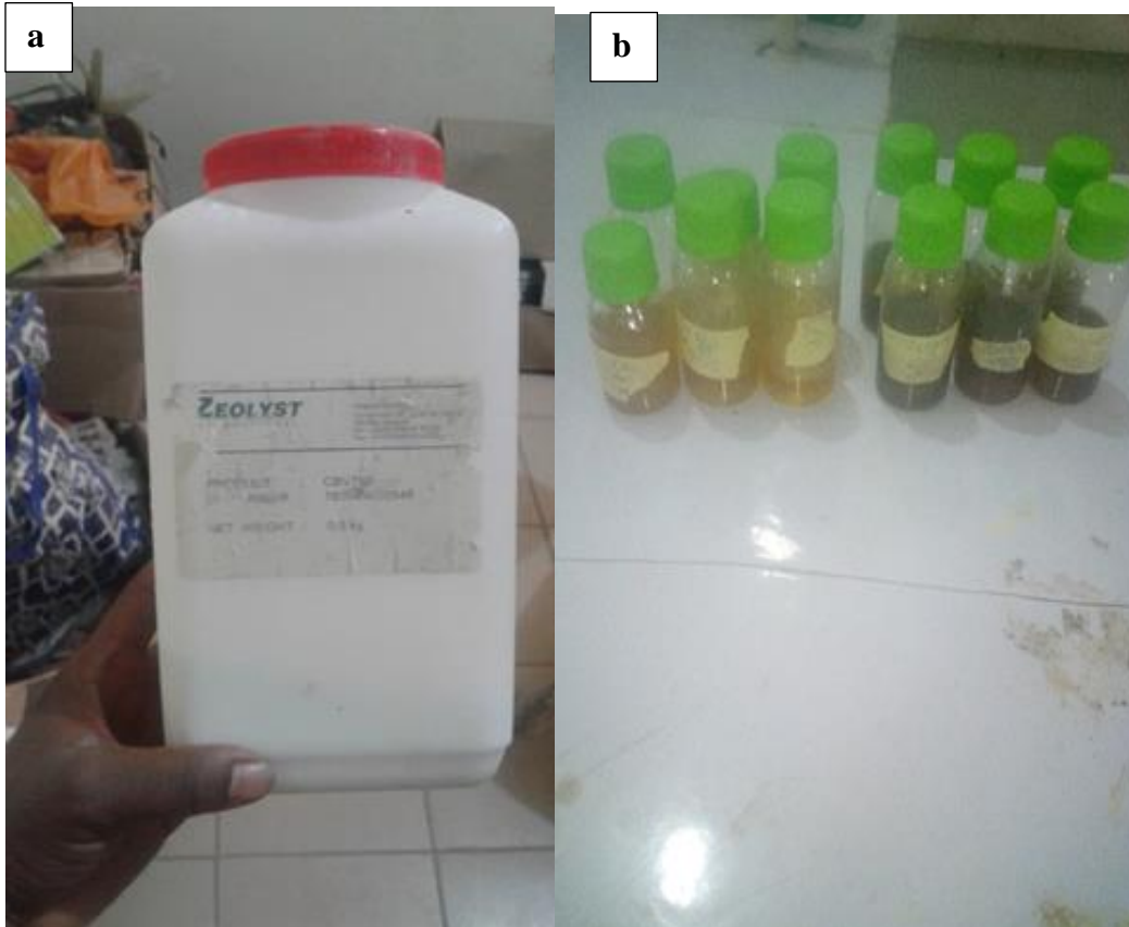
Plate D.4: (a) Zeolite Catalyst and (b) Pyrolysis Liquid Product
