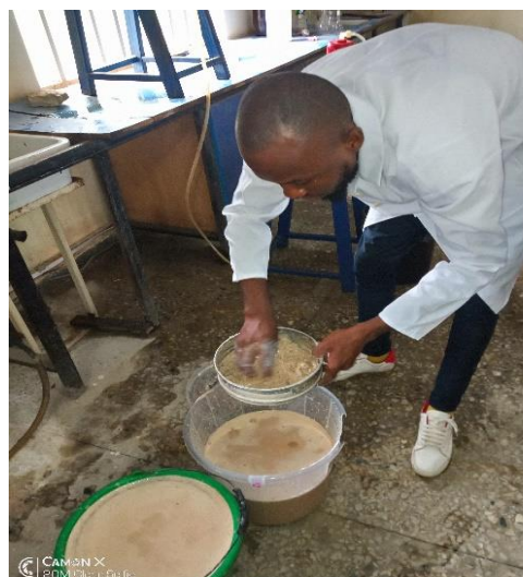
Plate VII: Beneficiation of kaolinite clay Plate VIII: Wet Sieving process
