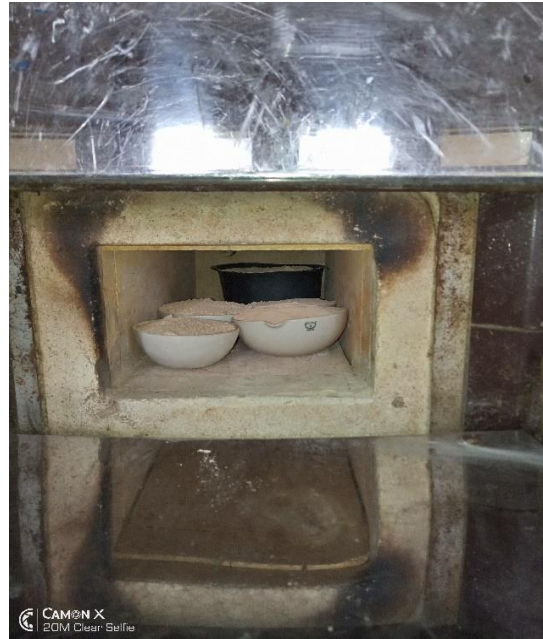
Plate X: Calcination of the beneficiated kaolin.
