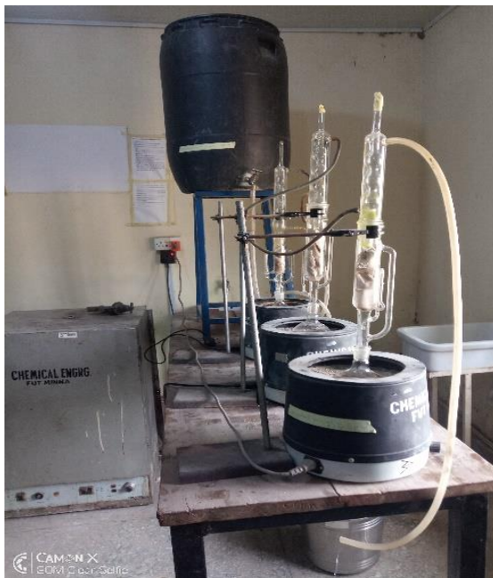
Plate V: Soxhlet extractor apparatus set
