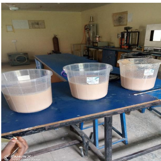
Plate VII: Beneficiation of kaolinite clay Plate VIII: Wet Sieving process
