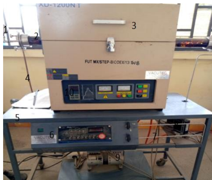
Plate II: Set-up of catalytic CVD for CNTs synthesis
