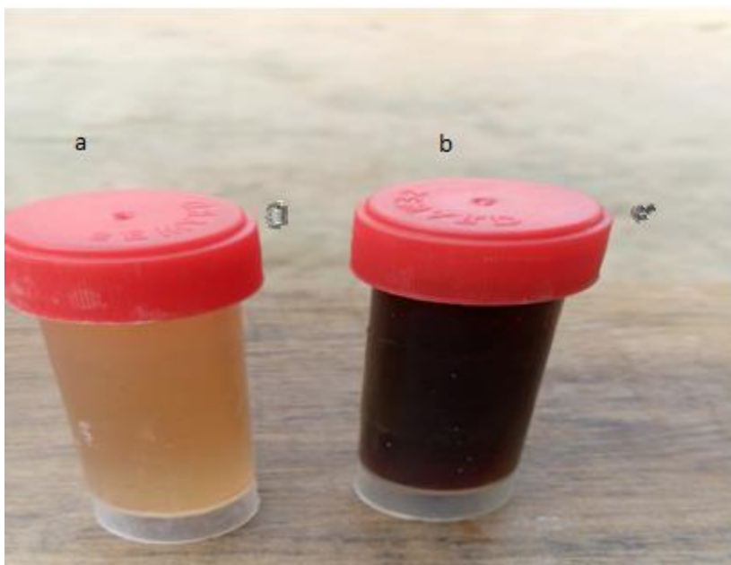
Plate IV: ( a) aqueous extract of pawpaw leaves (b) AgNPs from pawpaw leaf extract.
