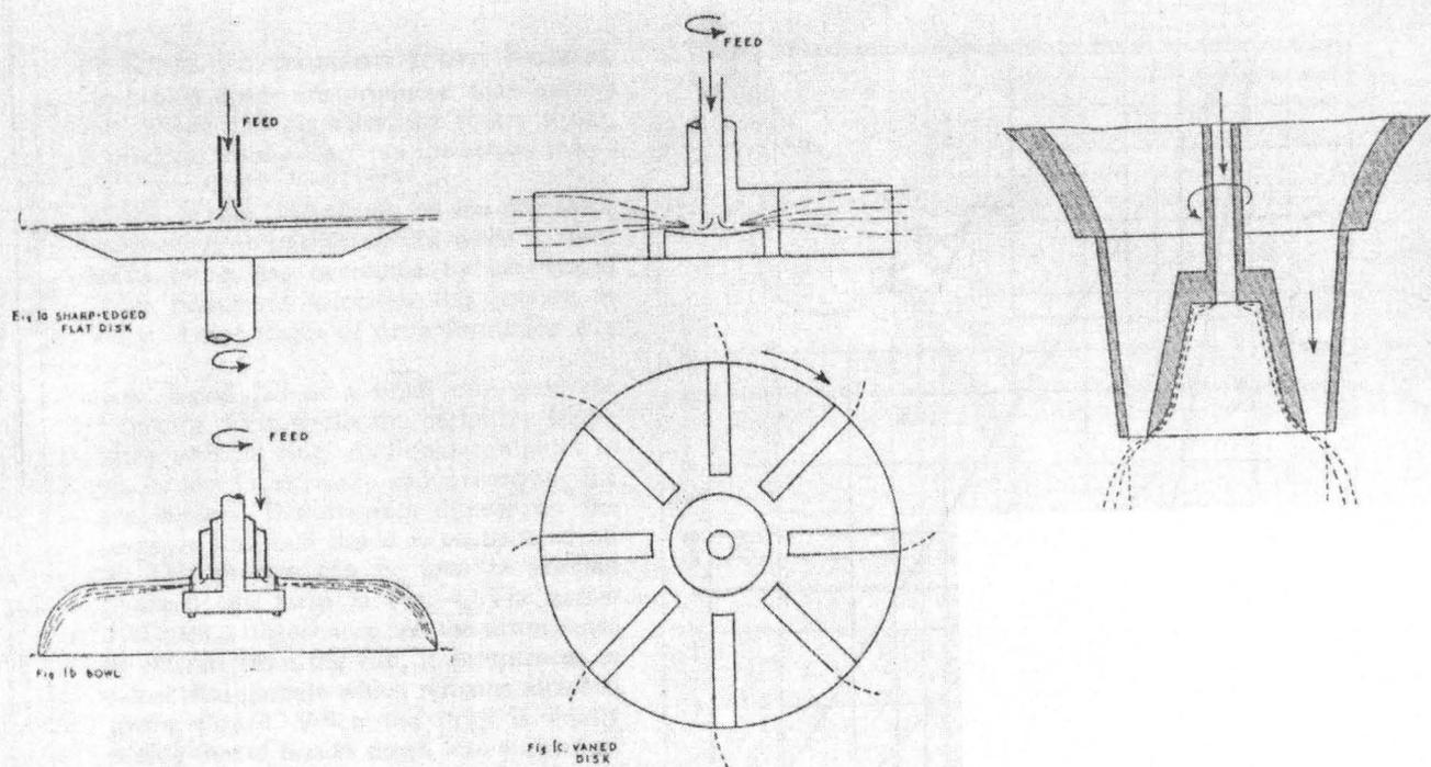
Figure 2.1 Characteristic rotary atomizers: (a) Sharp-edge flat disc; (b) Bowl; (c) Vaned disc; and (d) Air-blast bowl atomizer. (Fraser, et al, 1957).
