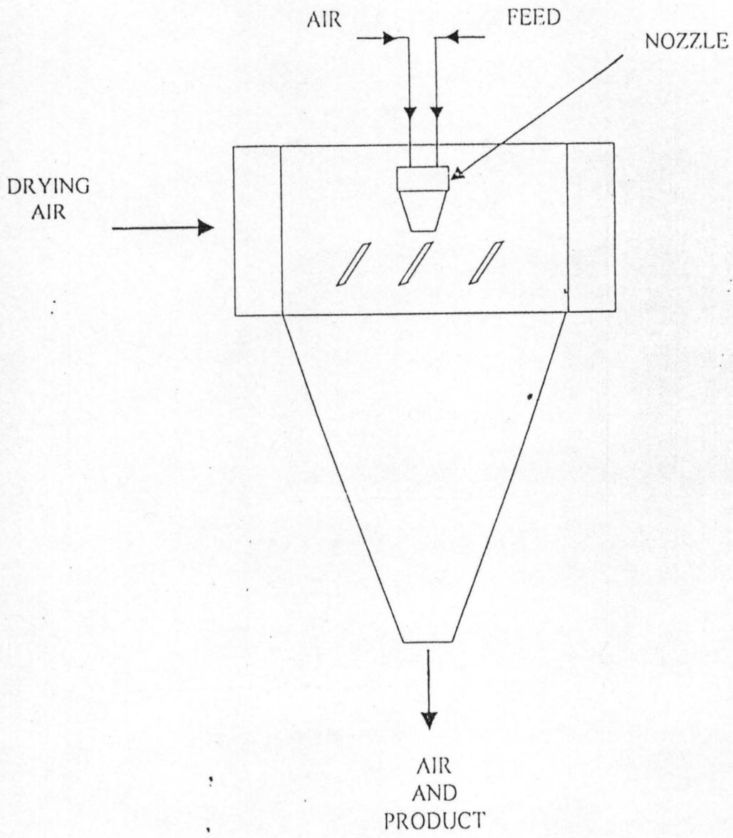
Figure 1.1 Schematic diagram of a typical spray dryer (Gauvin and Katta, 1975).
