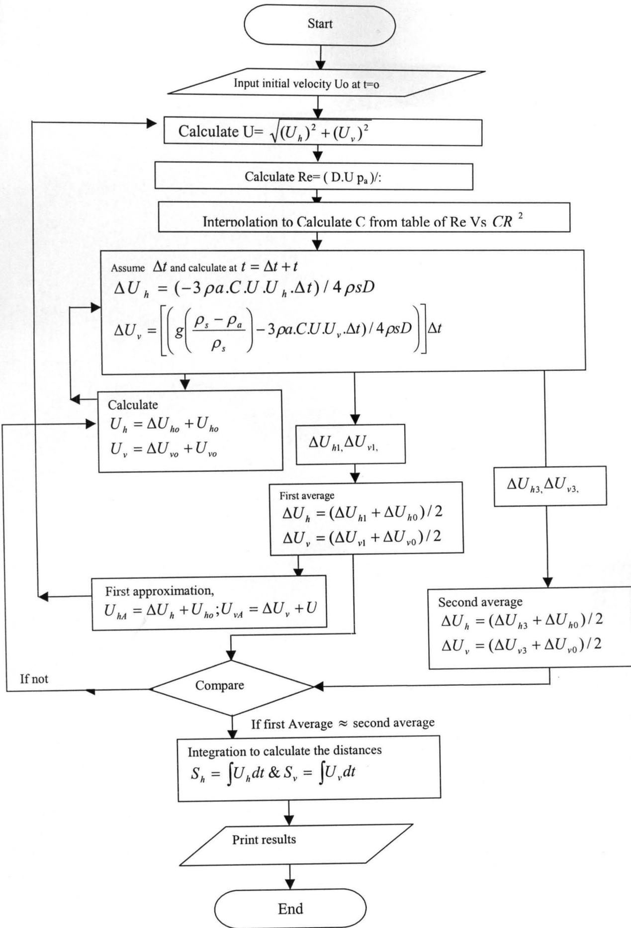
Fig. 3.2 A Flowchart of the program for Solving the equation of motion
