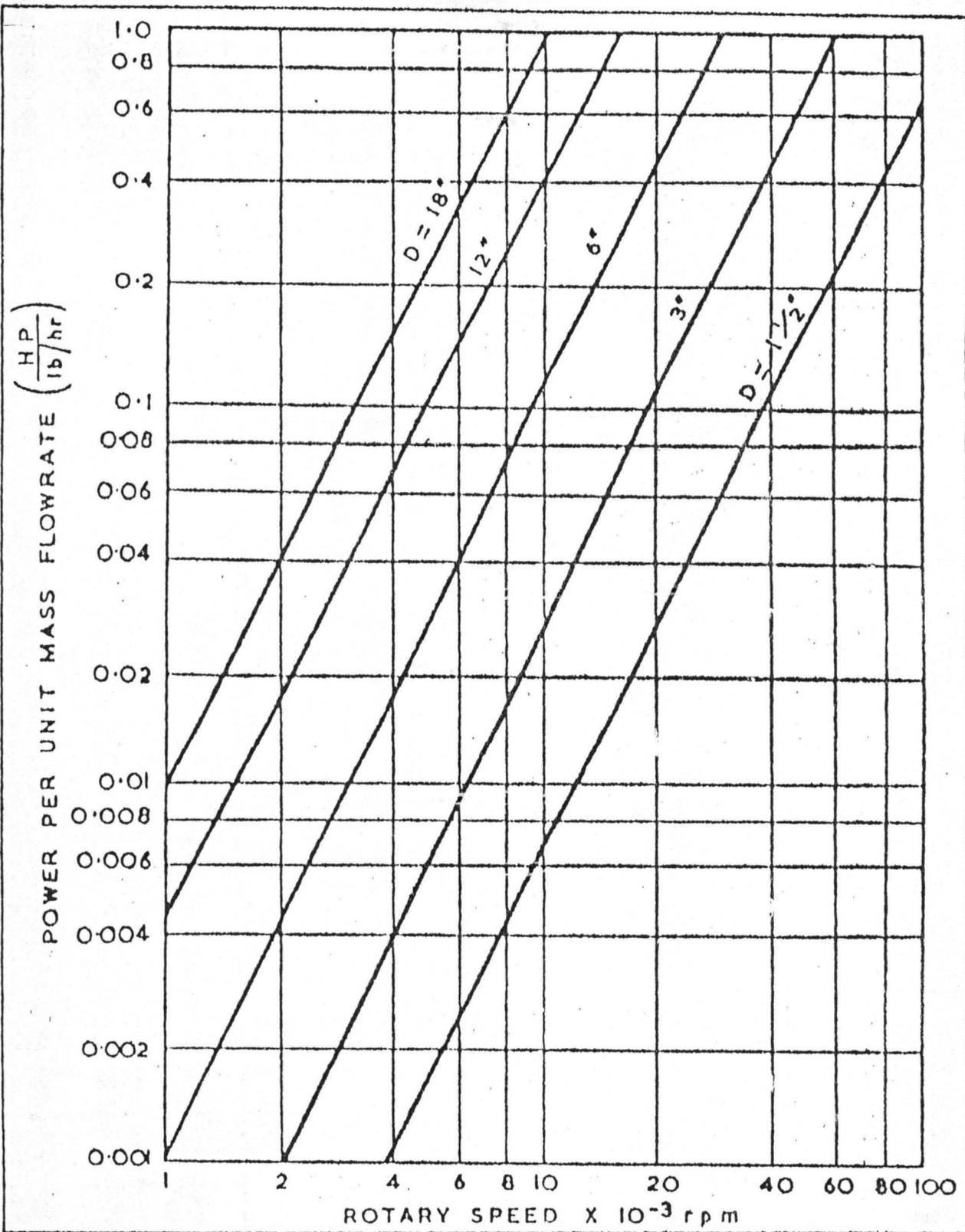
Figure 2.2 Theoretical power requirements above no-load conditions for various diameter discs and rotary speeds ( Fraser, et al, 1957).
