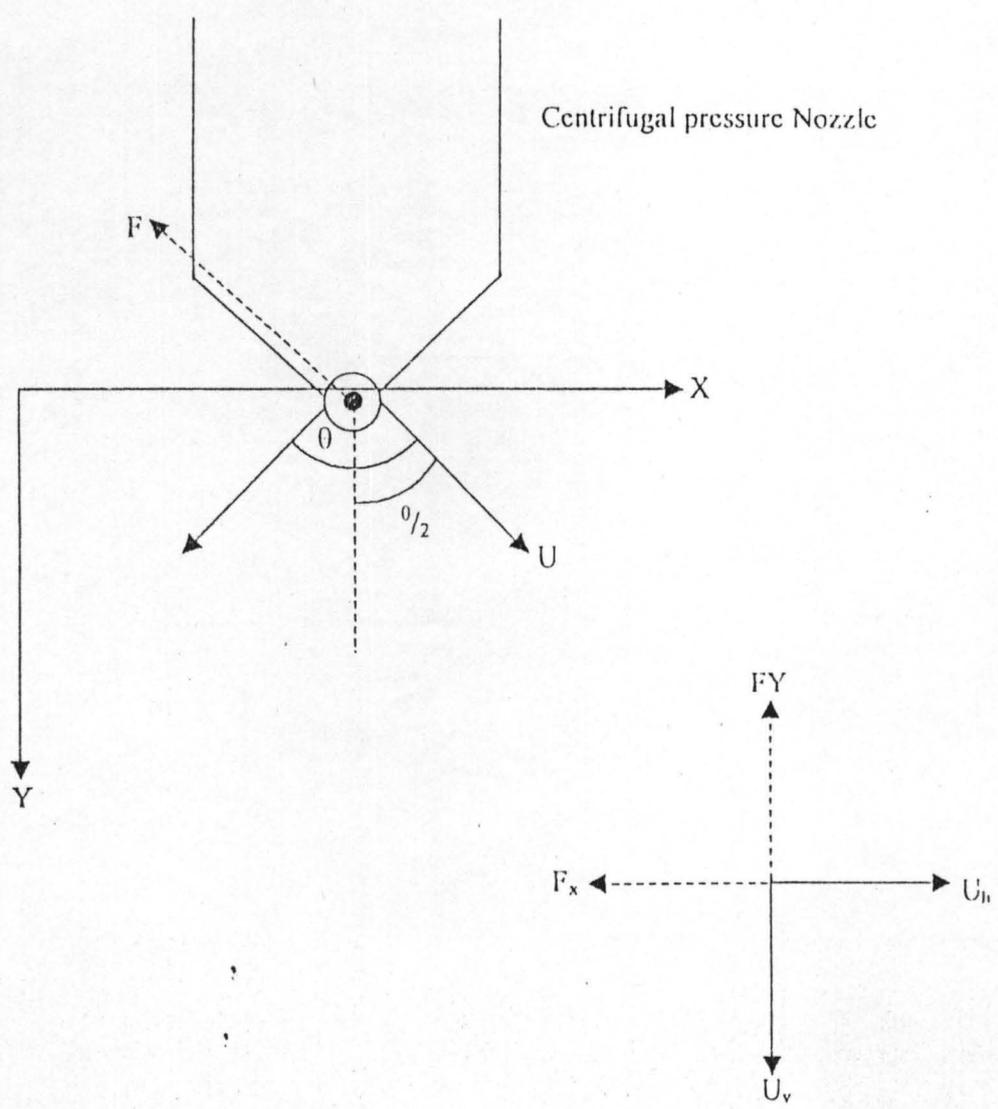
Figure 3.1 Force diagram for droplet trajectory
