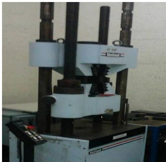
Plate IV: Tensile testing machine (UNITED type)
