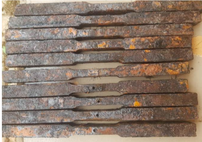
Plate XVI: Corroded Tensile Samples
