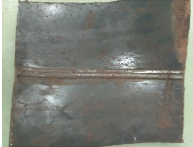
Plate XI: Welded API X70 steel plate
