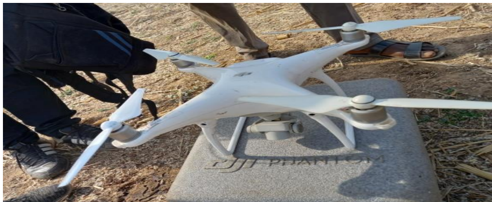
Plate II: Unmanned aerial vehicle DJI phantom 4
