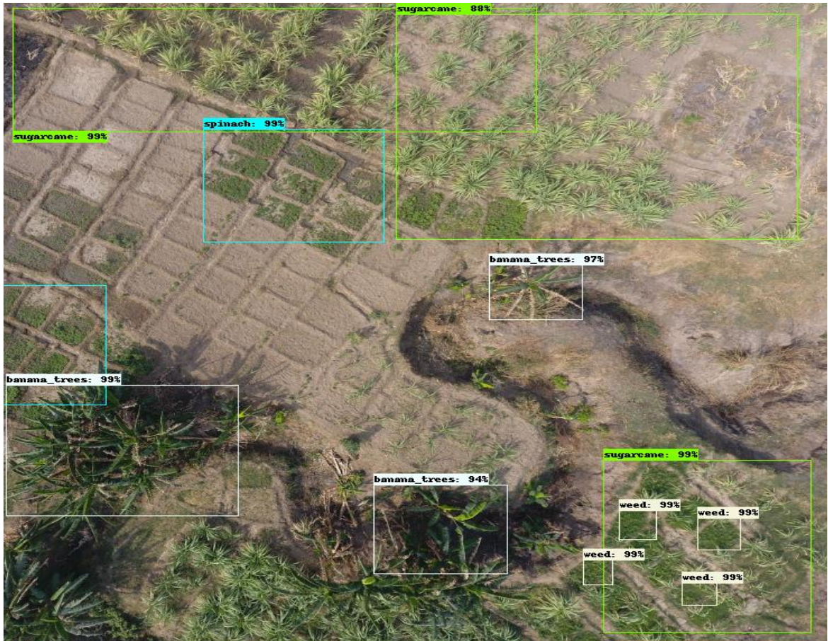
Plate VIII: The classifier's confidence in detecting and classifying weed classes was 99 % in accuracy at 200,000 epochs from the image
