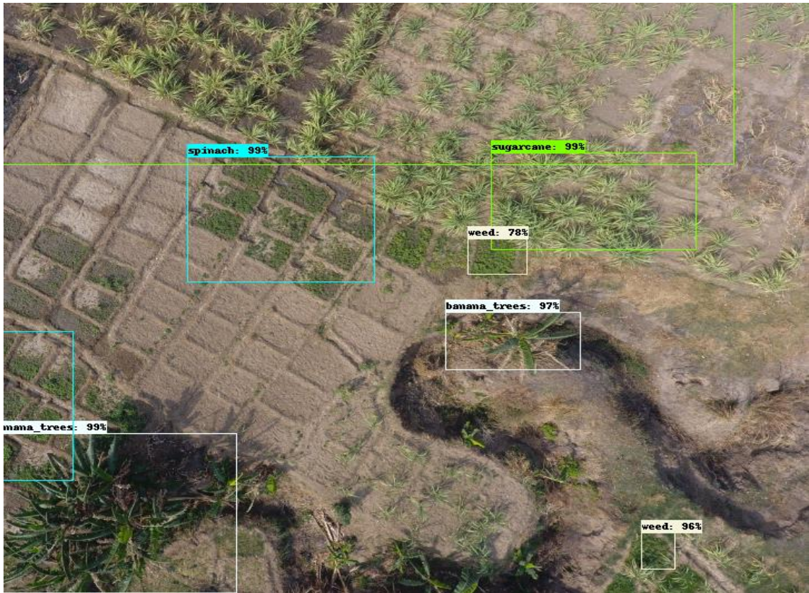
Plate IX: The classifier's confidence in detecting and classifying weed classes was 96 % in accuracy at 242,000 epochs from the image
