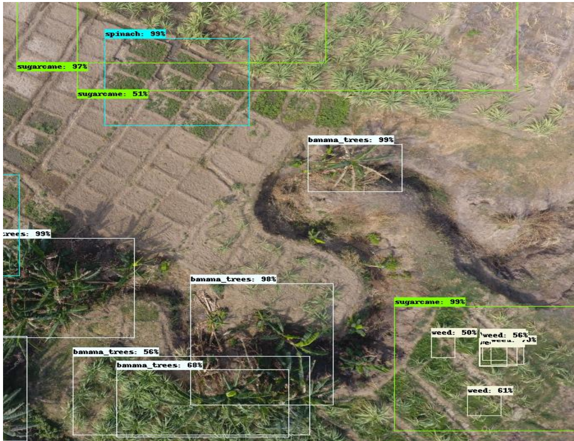
Plate VI: The classifier's confidence in detecting and classifying weed classes was 67 % in accuracy at 20,000 epochs from the image
