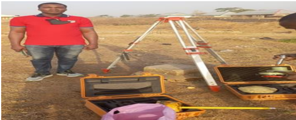
Plate IX: The DGPS instrument used for acquiring GCP's
