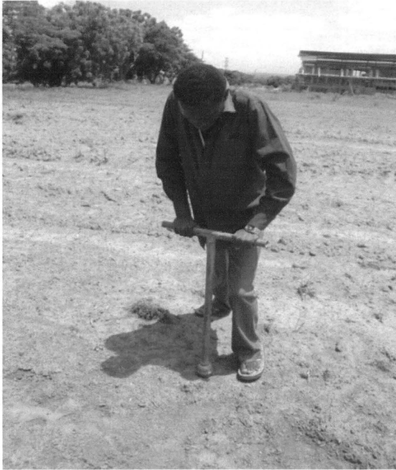
Plate 3.8 Picture Showing the Collection of Soil Sample Using the Bulk Density Apparatus
