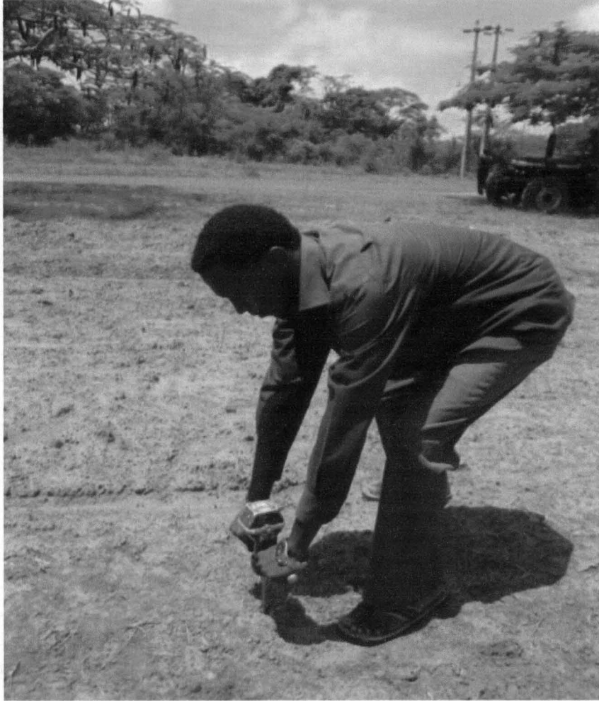
Plate 3.6 Picture Showing the Measurement of Cone Index Using the Cone Penetrometer
