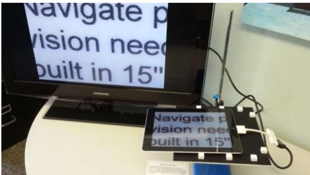
**Figure 2.3 Magnification system**
