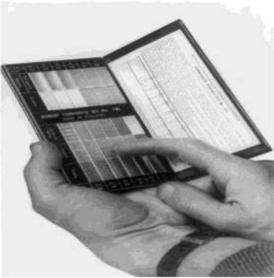
Figure 4.25: Surface roughness comparison specimens
