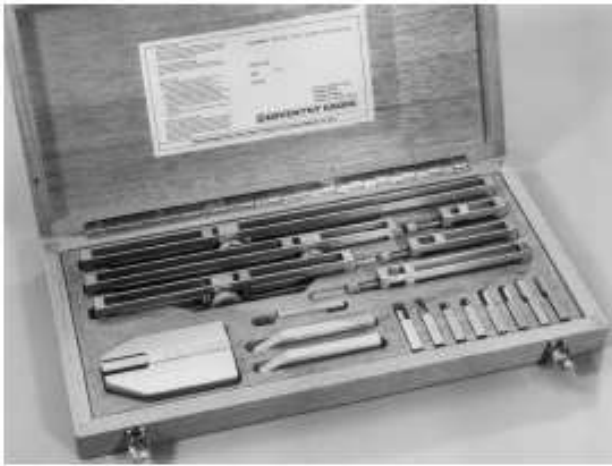
Figure 4.5 Set of gauge-block accessories
